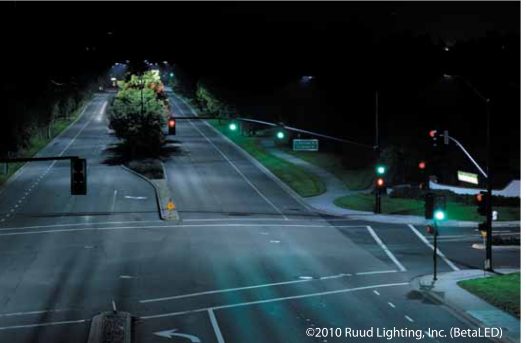
LEDway streetlight with 60 LEDs, Type III medium optics, 525mA, Color Temperature: 6000K
